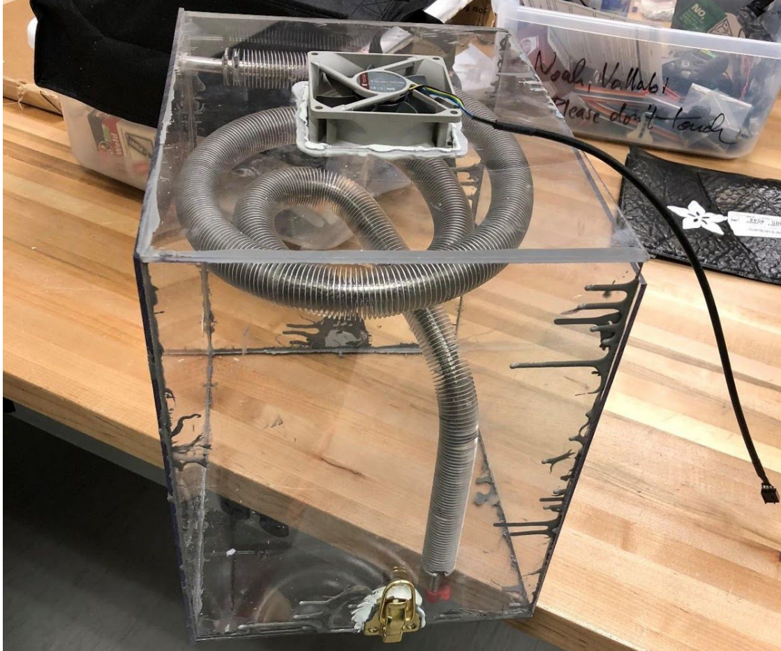
Figure 1: This image shows the completed second chamber. The fan at the top will be used to cool the inside of the chamber down as the condenser coil lowers the temperature of the water vapor. The tops of the latches can be seen on the sides of the chamber, towards the bottom; these latches will be used to secure the water storage container securely in place.
