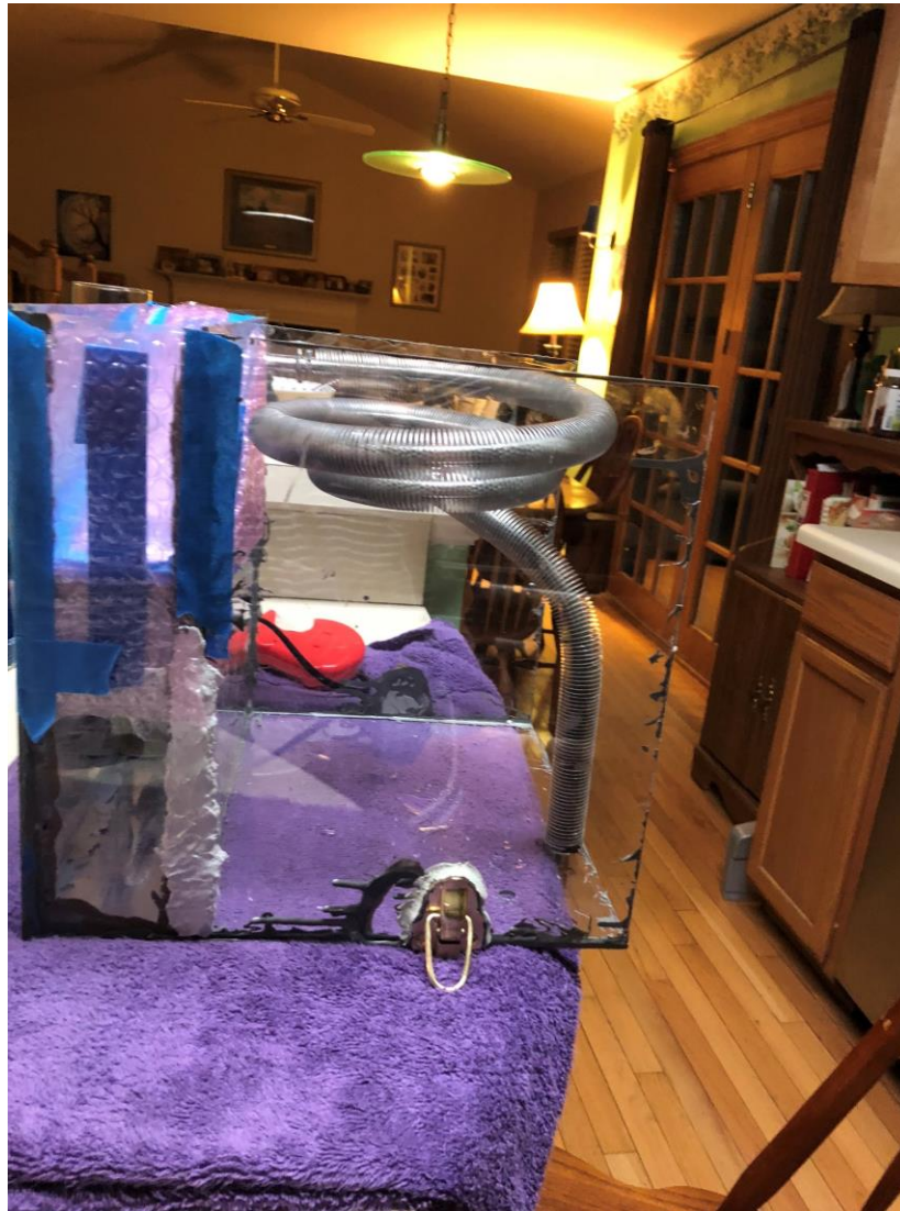
Figure 1: This image shows the insulation that was placed around the first chamber to prevent condensation on the inside.
