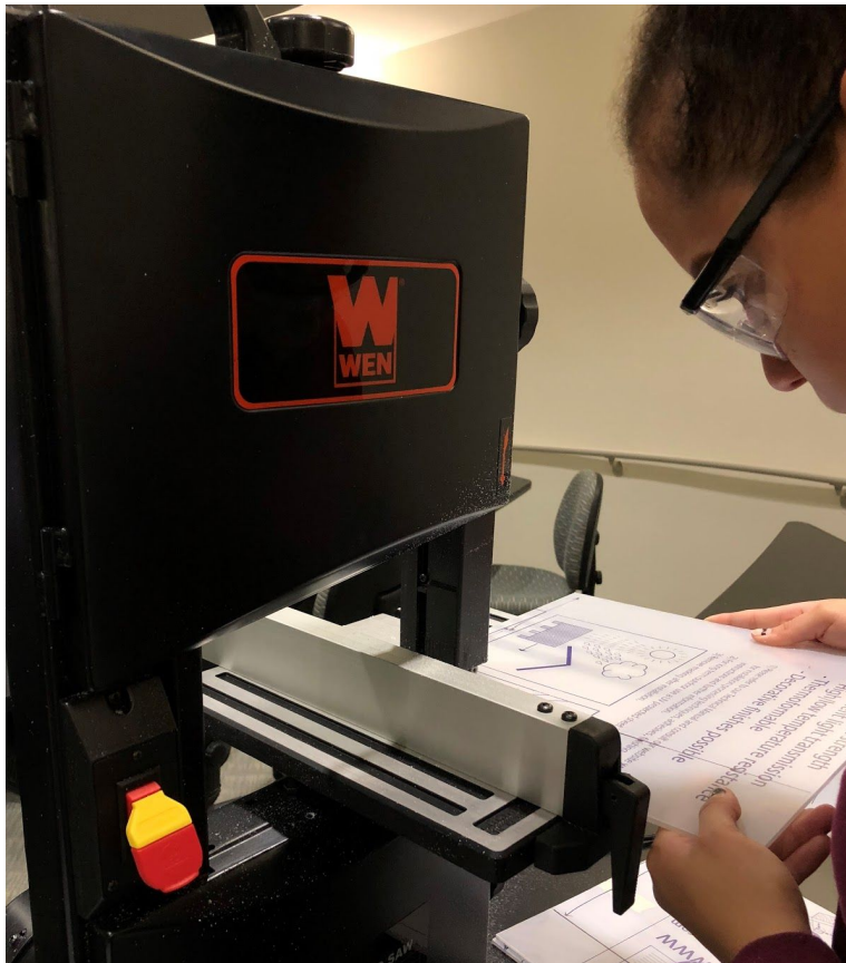
Figure 3: This image shows the plastic being cut by the band saw. This was a first time experience of using a band saw, and it proved very helpful and simple for cutting the polycarbonate plastic.
