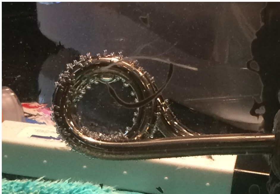
Figure 1: This shows the water heater after one minute of operation. The bubbles on the heater show that the water is heating, not reaching a boiling point yet, but close none the less.
